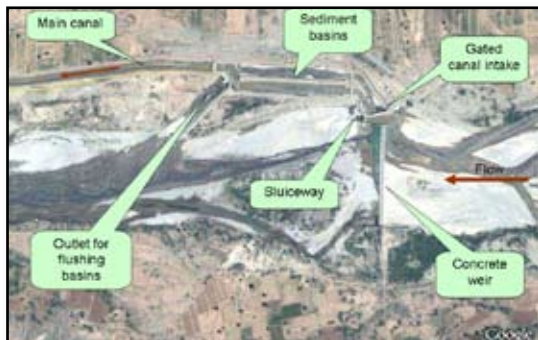
Figure 10. Typical conventional diversion structure
