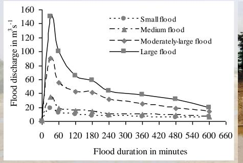
Shift to individual field distribution system? Large spate flows in short period Sediment control and management Field-to-field: reduce command area
