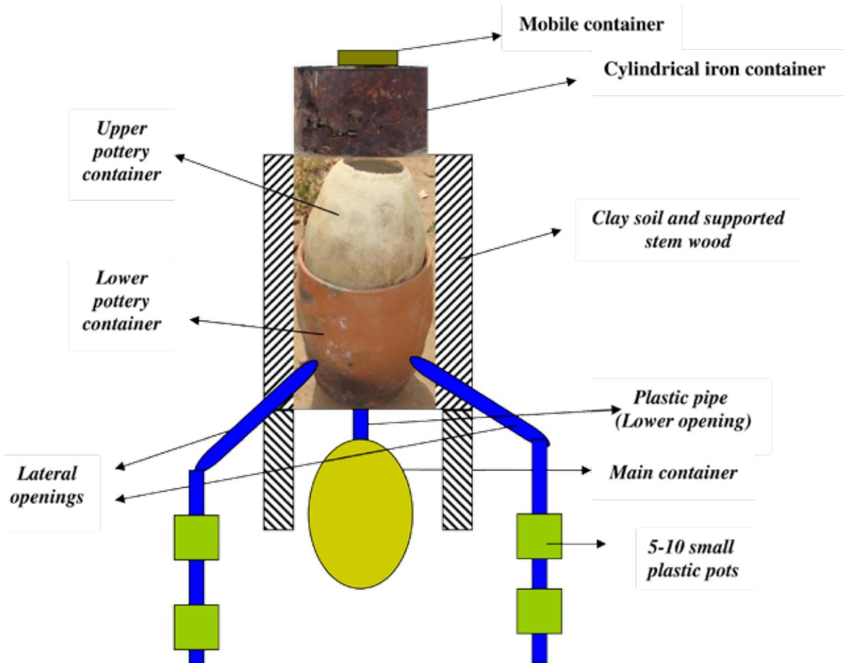
Figure 11 Schematic overview of the *qataran* extracion device
