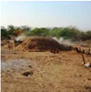
7. Ignite the pile through 1-2 small openings
