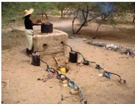
Figure 10 Typical *qataran* extraction device.
