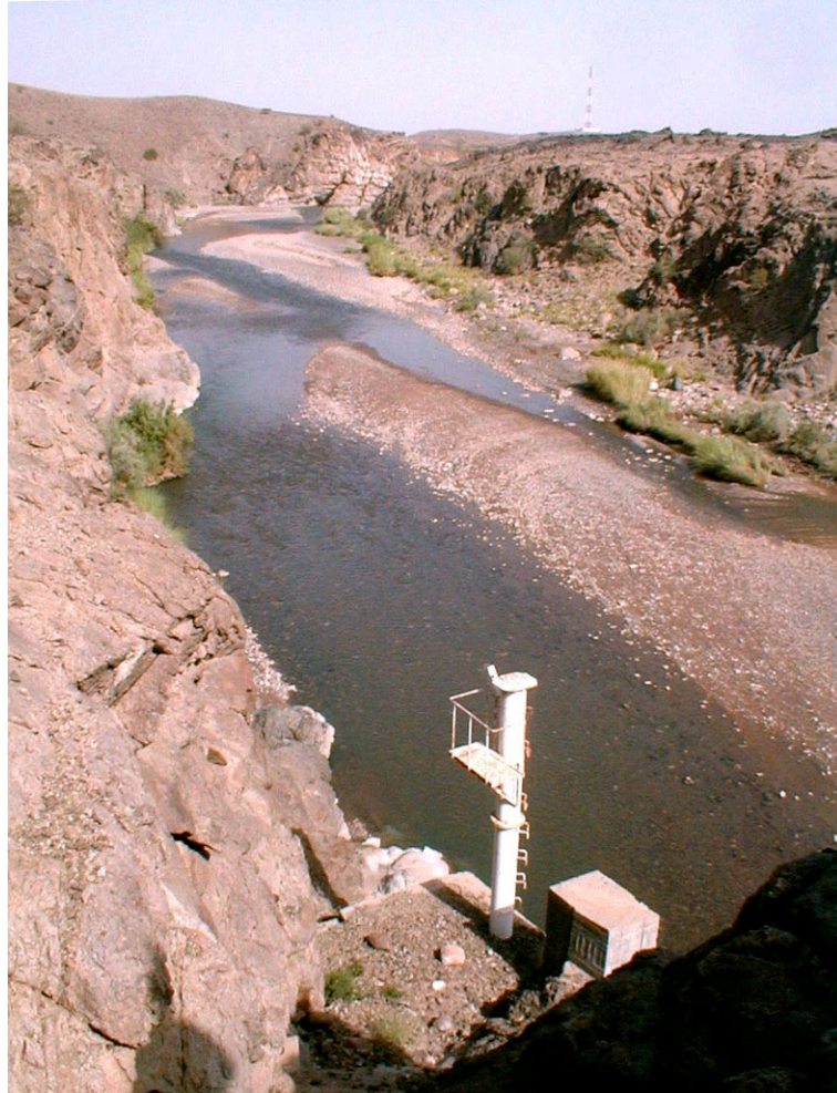
Figure 4.4 Wadi stream gauging site located in a gorge section close to the mountain front, Wadi Tuban, Yemen.
