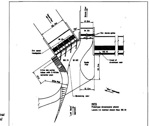
Figure 5 General layout of headworks for model tests
