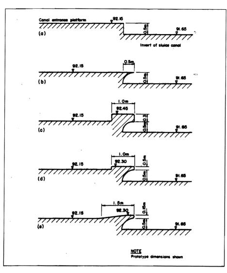
Figure 6 Skimming weir details for different models
