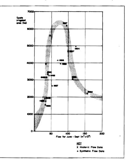
Figure 1 Relationship between wadi flows and irrigated areas from analysis of Zakat records engines. The state farm at Wadi Surdud was an exception with a central generating station supplying power to submersible pumps in the boreholes.
