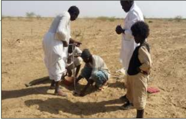
collecting soil sample using hand-auger
