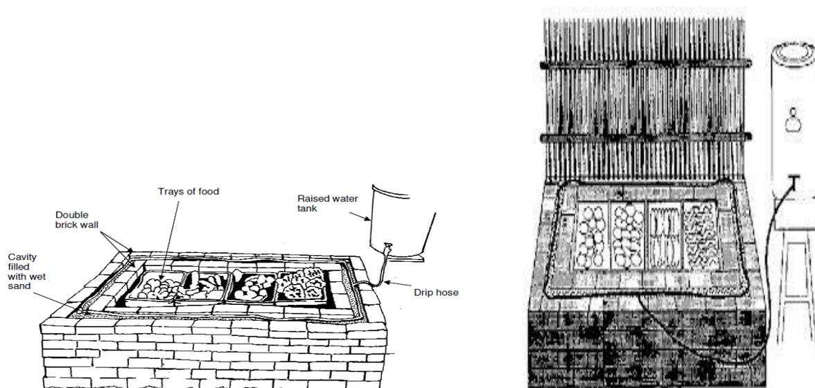
Fig 18: Static cooling chamber
