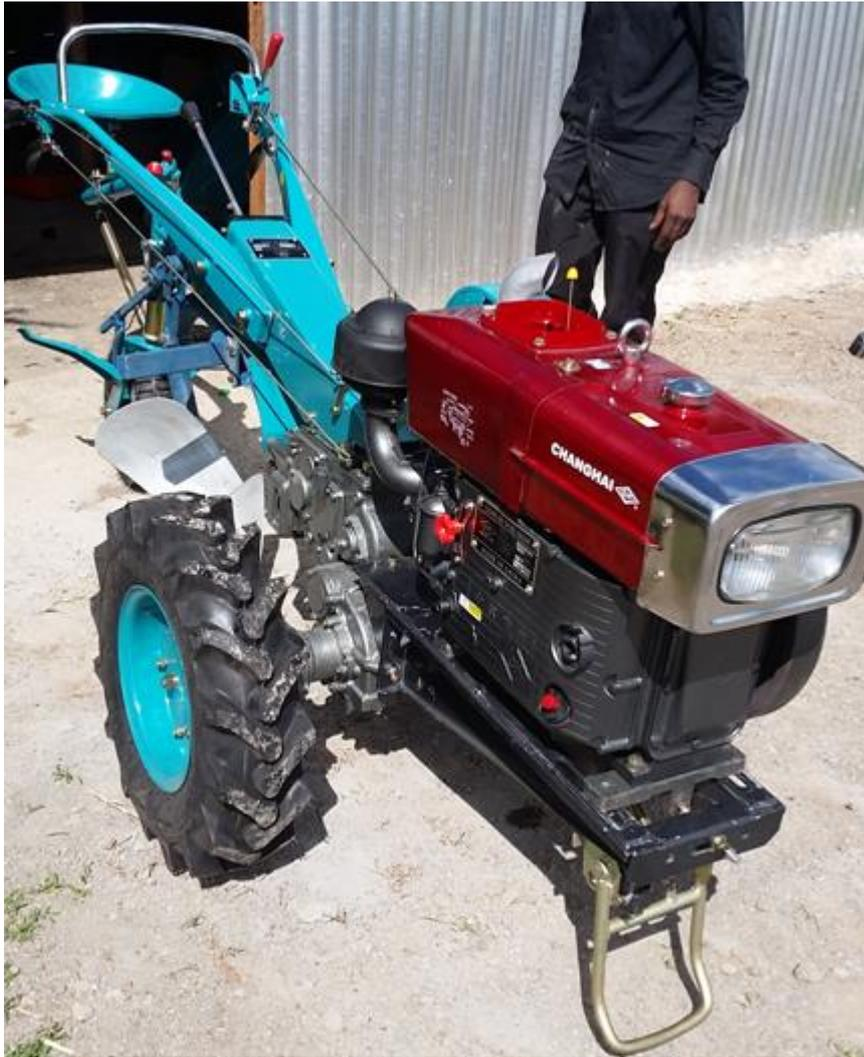
*Fig 14: Single Axle Tractor*
