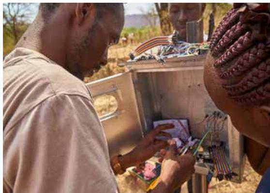
Figure 2: Connection of the moisture sensors to the board
