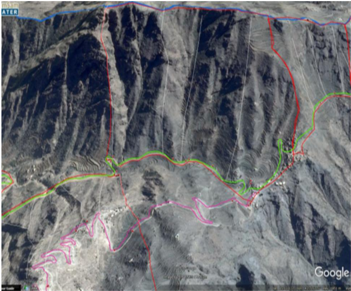
Figure 67 a sample of the road natural catchment area which is calculated by Google-Earth tool
