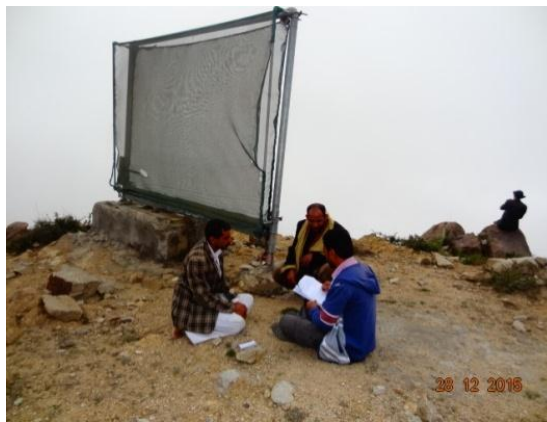
Figure 8 Fog harvesting unit (pilot project by UNDP’s (WGP-AS)
