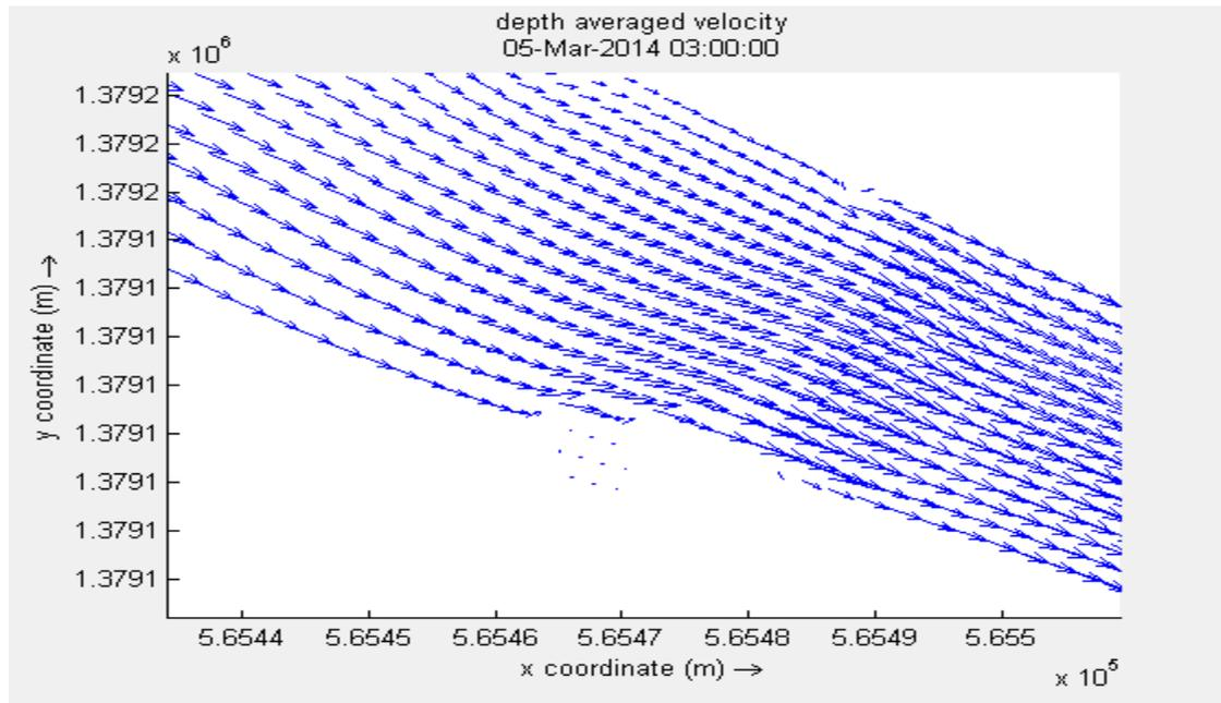
**Figure 6.5** Flow patterns of the flood for scenario one
