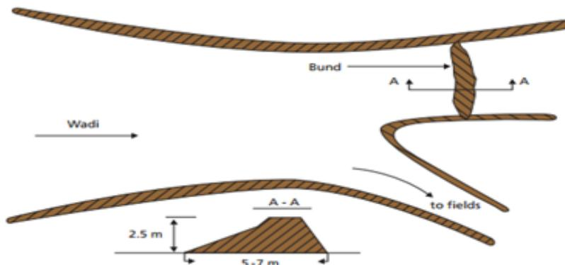
**Figure 3.4** Bund type traditional intake (Source: adopted from Van Steenberg et al., 2010)
