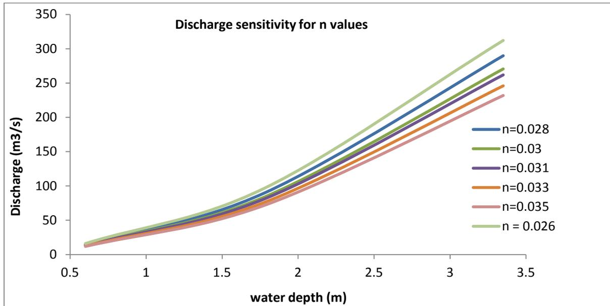
**Figure 4.6** Discharge sensitivity at different values of roughness coefficient (n)
