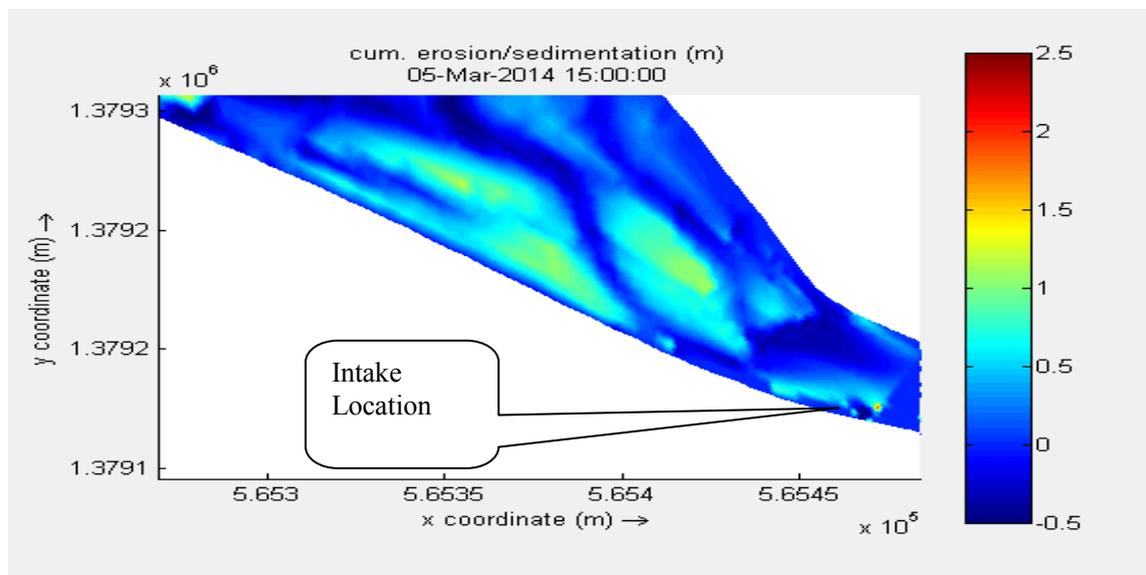
Figure 6.16 Cumulative erosion/sedimentation scenario four
