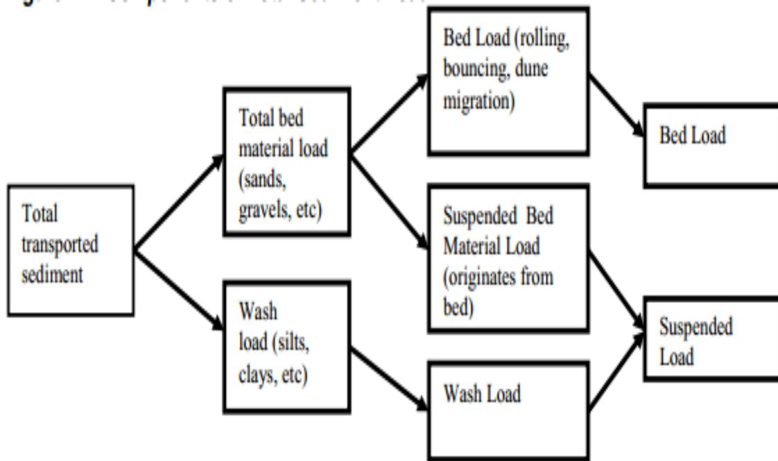
**Figure 3.5** Components of total sediment load (source Ratsey, 2011)
