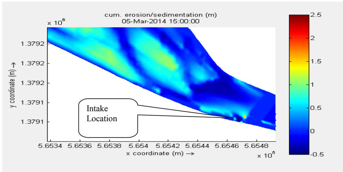
Figure 6.13 Cumulative erosion/sedimentation scenario three
