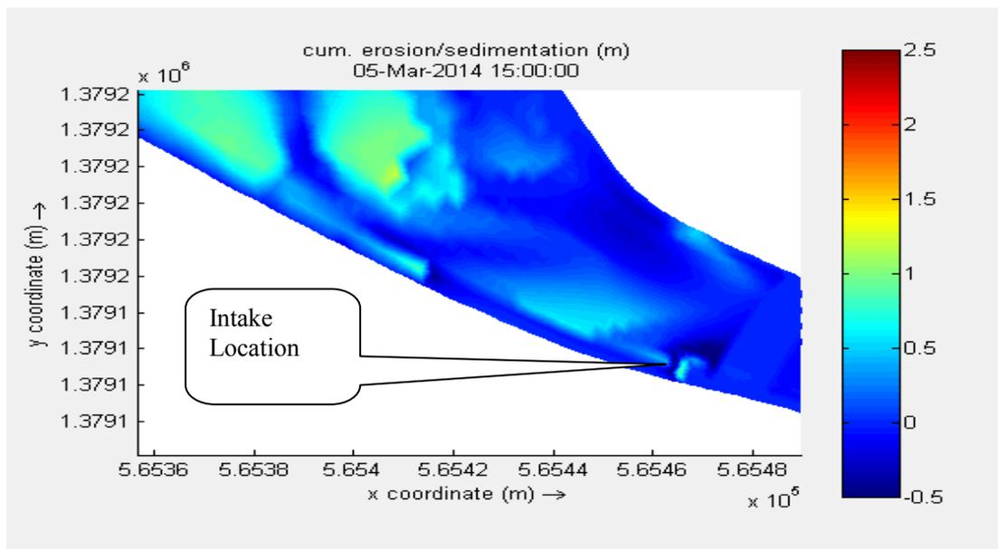
Figure 6.7 Cumulative erosion/sedimentation scenario one
