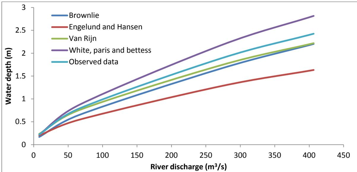
**Figure 4.8** Comparisons of depth estimates from different alluvial friction predictor of DORC model
