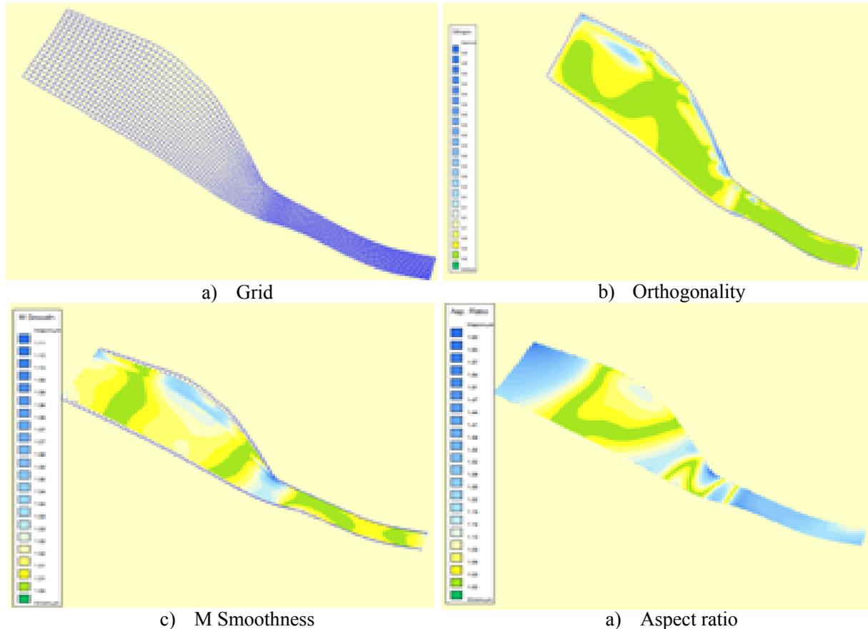
**Figure 5.1** Grid development and grid properties
