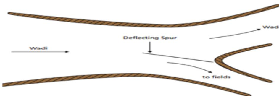
**Figure 3.3** Deflecting spur type traditional intakes (Source: adopted from Van Steenberg et al. 2010)
