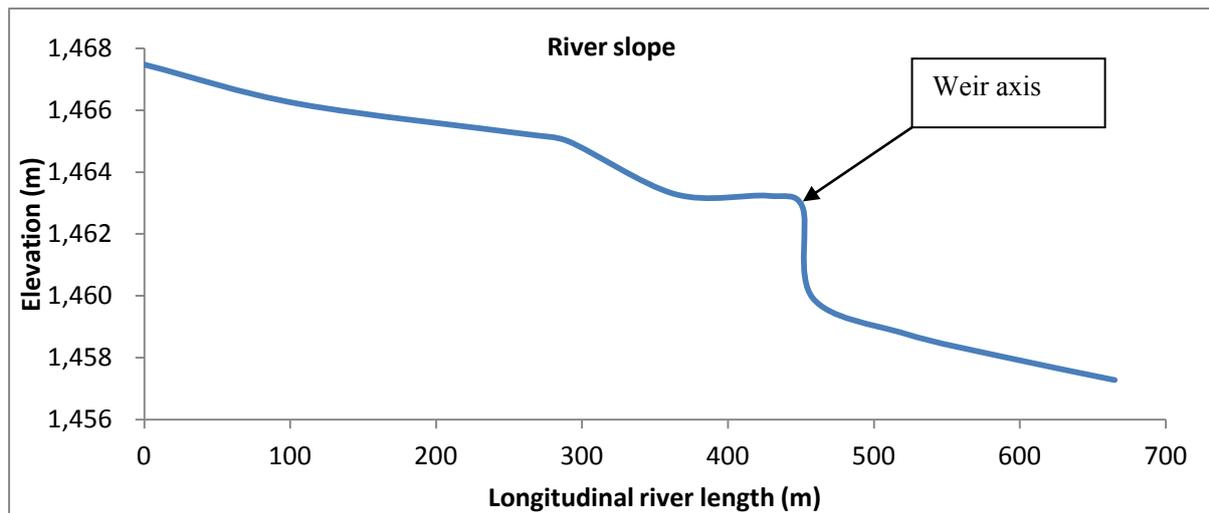
**Figure 4.2** River bed slope in longitudinal direction (not in scale)
