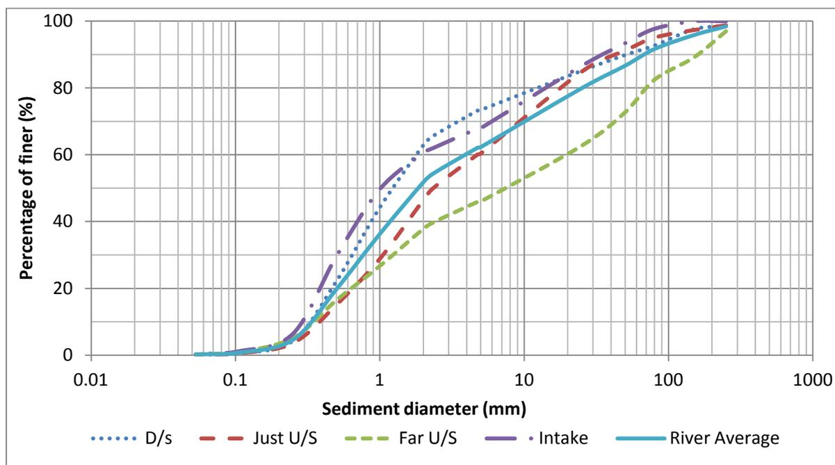
**Figure 4.5** Sediment grading graph at different cross sections of the river
