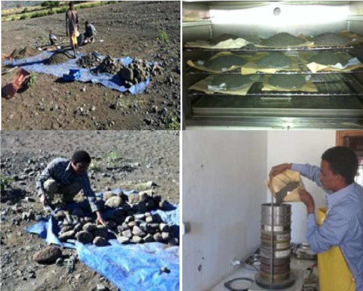
**Figure 4.4** Sediment bed material grading manual sieving at field (left) and mechanical sieving at laboratory (right)
