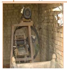
The fodderc hopper is a hand or electricity driven machine that can be used to chop fodder. It saves time and energy compared to manual cutting of fodder and is easy to maintain and operate. It can be adjusted to chop dry and fresh fodder and can be produced locally.
