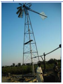
A Windmill that converts wind into energy to pump irrigation water.
