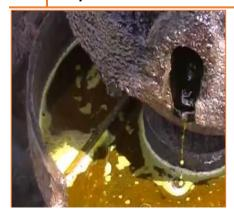
The oil press is an electrical machine that extracts oil from different kind of seeds such as rapeseed, mustard and sesame. It processes the seeds to produce a high value oil and reduces potential losses from rodents, birds and molds attacking seeds. The raw seeds are squeezed under high pressure, friction causes it to heat up and the oil seeps through small openings that do not allow seed fiber to pass.
