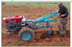
The single ale tractor is powered by a fuelefficient water-cooled diesel engine and can be fitted with metal paddle wheels for working in wet conditions to prevent slipping. The machine is able to undertake multitask agricultural operations like ploughing, rototilling and towing trailer. In stationary mode as a power source it can be used for water pumping, grain threshing, flour milling, fodder cutting and food oil pressing.
