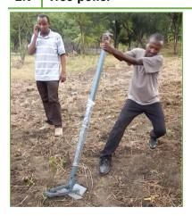
The tree puller is used to uproot small trees or old trees and has a claw, fulcrum and an arm as lever with which trees with a stem diameter up to 5cm and with relatively shallow rooting systems can be uprooted.
