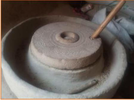
*A flour mill is a mechanical grinding machine used to make flour by rotating two stones. It has a bigger capacity and conserves more time and energy for operating as compared to a hand flour mill. It can be locally produced.*
