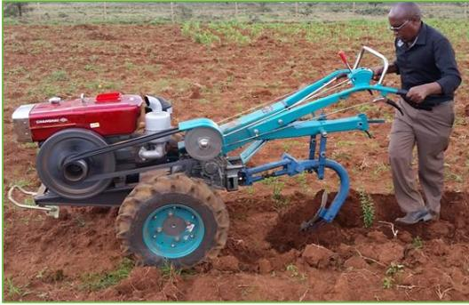
*The single axle tractor is powered by a fuel-efficient water-cooled diesel engine and can be fitted with metal paddle wheels for working in wet conditions to prevent slipping. The machine is able to undertake multitask agricultural operations like ploughing, rototilling and towing trailer. In stationary mode as a power source it can be used for water pumping, grain threshing, flour milling, fodder cutting and food oil pressing.*
