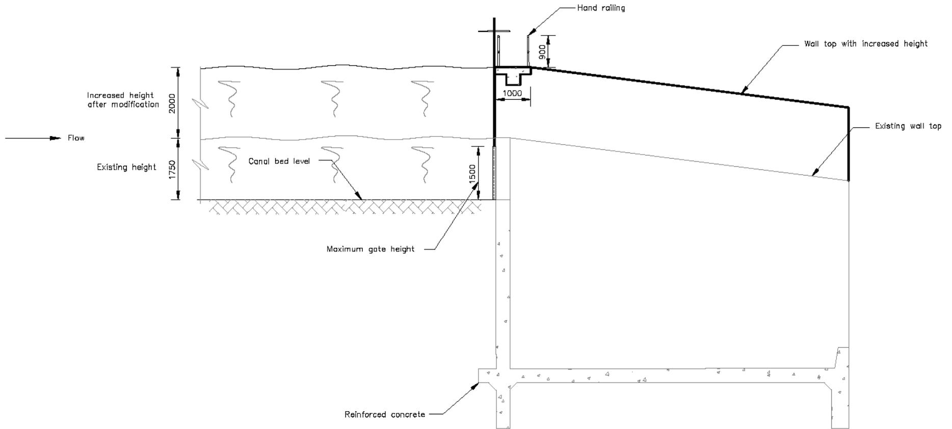
**Drawing 7: Section Through Modified Drop Structure**
