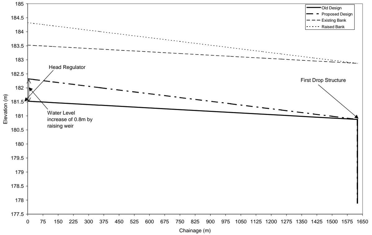
**Drawing 4 - Modified Cross Section With Reduced Drop Height**
