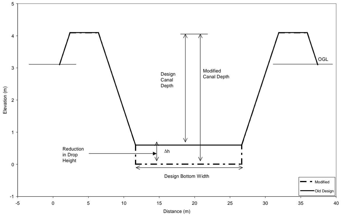
**Drawing 5 Modified Cross Section With Raised Weir Crest Level**
