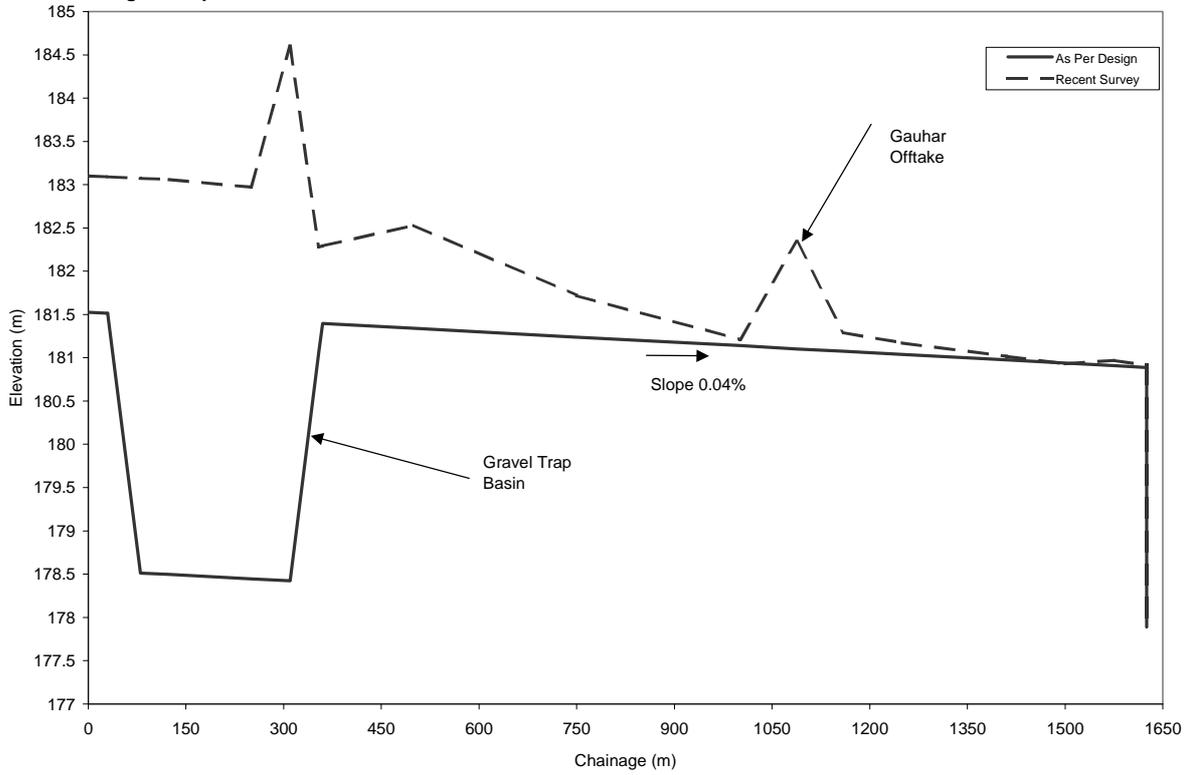
**Drawing 2 - Head Reach Remodelling With Drop Height Reduction - Longitudinal Profile**
