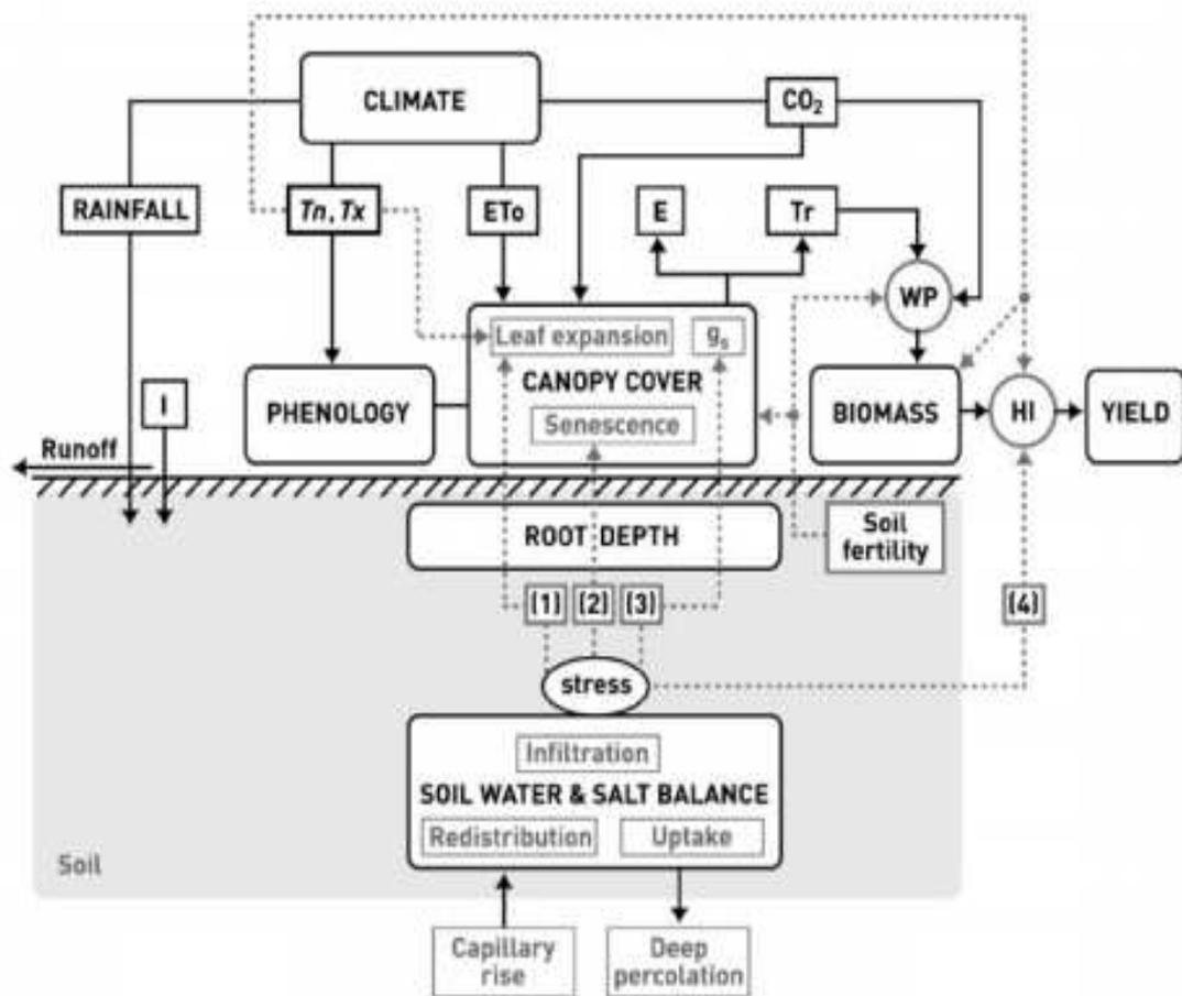
**Figure 2.3** Main components of soil-plant-atmosphere
