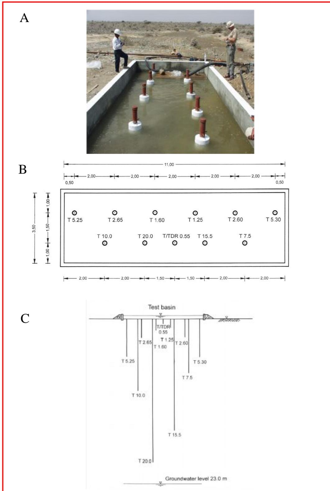
Figure 2.3 (A) Photo of test basin (B) Layout of the test basin (C) Vertical cross section of the test basin and subsoil. (Zunic, *et al.*, 2001).
