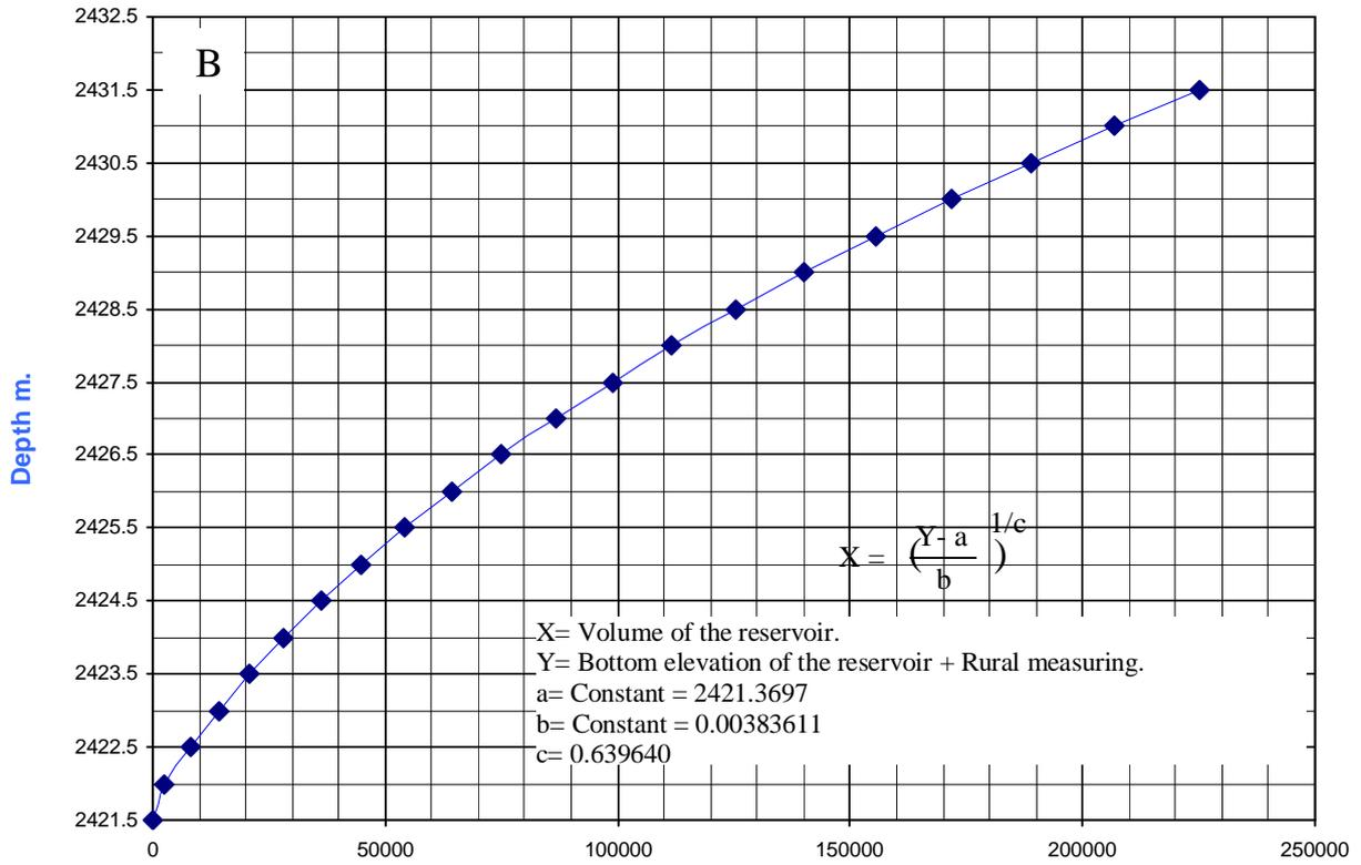
Figure 3.5 (B) Curve for calculation of reservoir's volumes (SBWMP, 2008)
