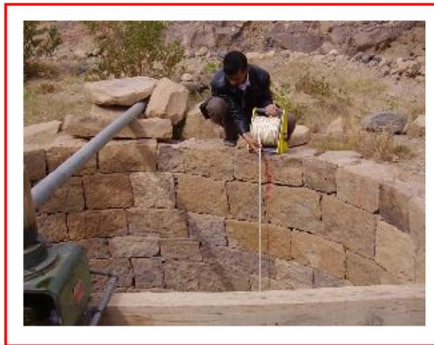
Monitoring wells water level by using Electric Sounder
