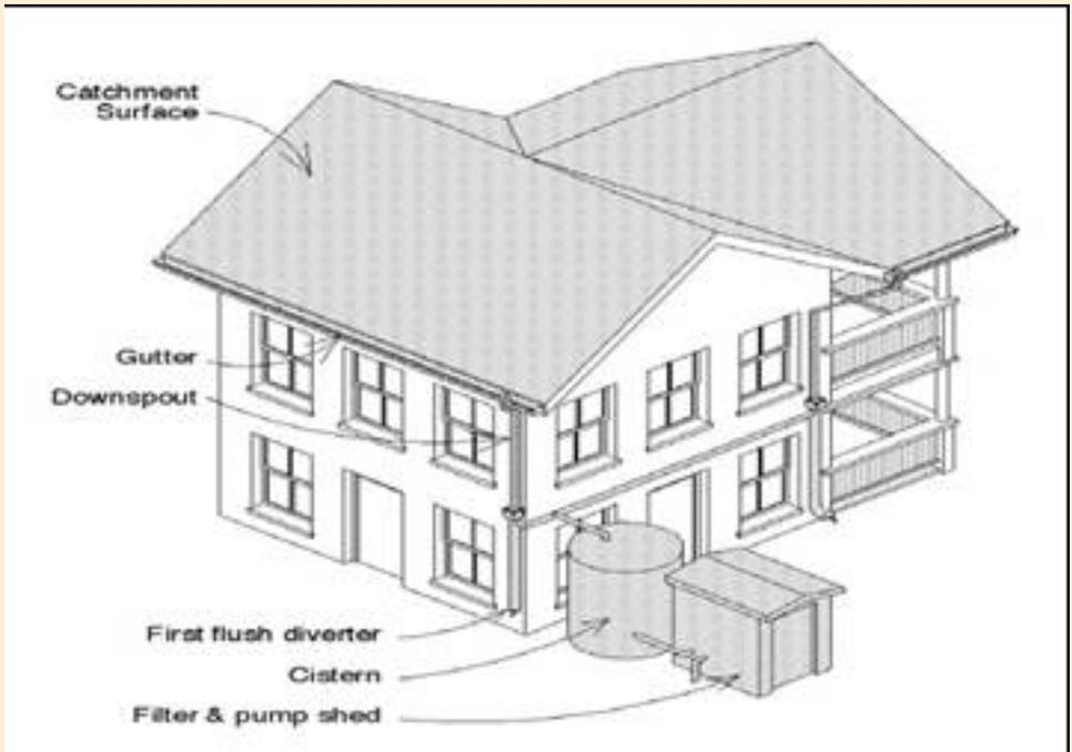
Figure (2.2): Roof catchment system [6]
