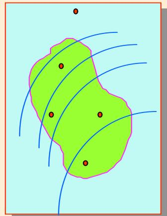
Figure (5.7): Draw the isohyetal lines
