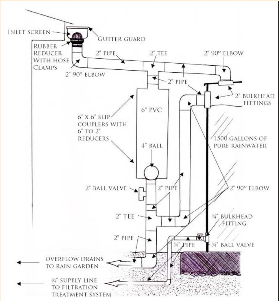
Figure (2.4): Basic rooftop water harvesting system including first flush pipe [7]
