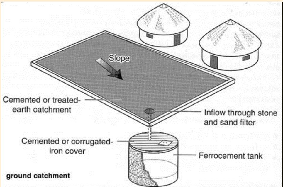
Figure (2.3): Ground catchment system [6]
