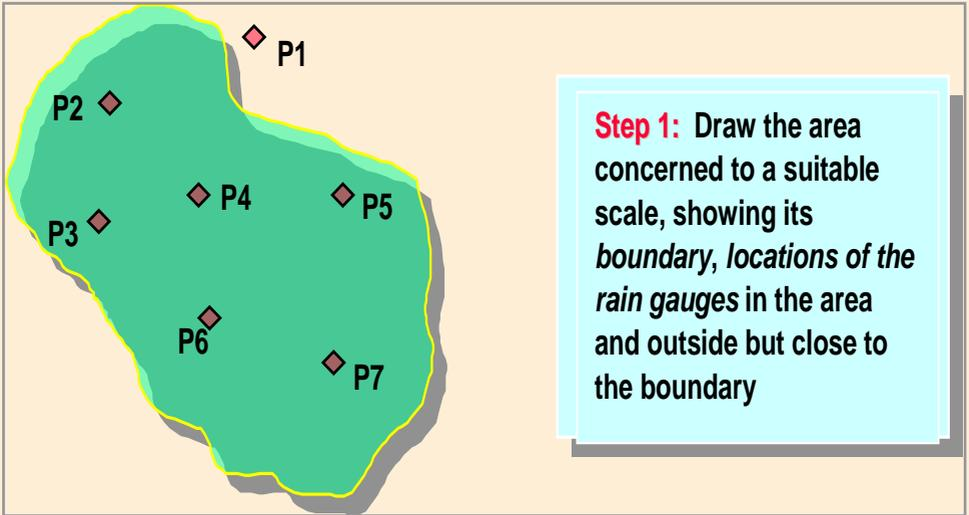
**Step 1:** Draw the area concerned to a suitable scale, showing its *boundary, locations of the rain gauges in the area and outside but close to the boundary*
