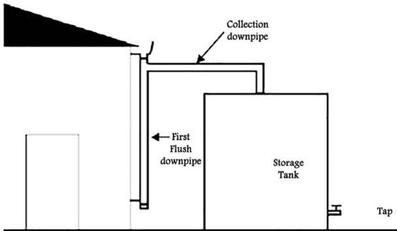
Figure (2.7): Semi-automatic Method: Simple down pipe first flush device [11]
