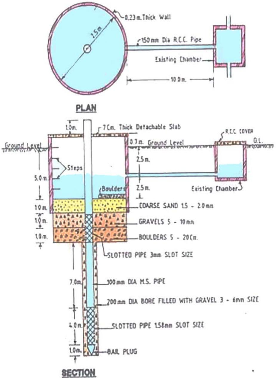
Figure (4.4): Chamber with tube well for ground water recharge [14]
