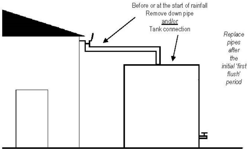
Figure (2.6): Manual Method: Simple downpipe manually moved away for first flush [11]
