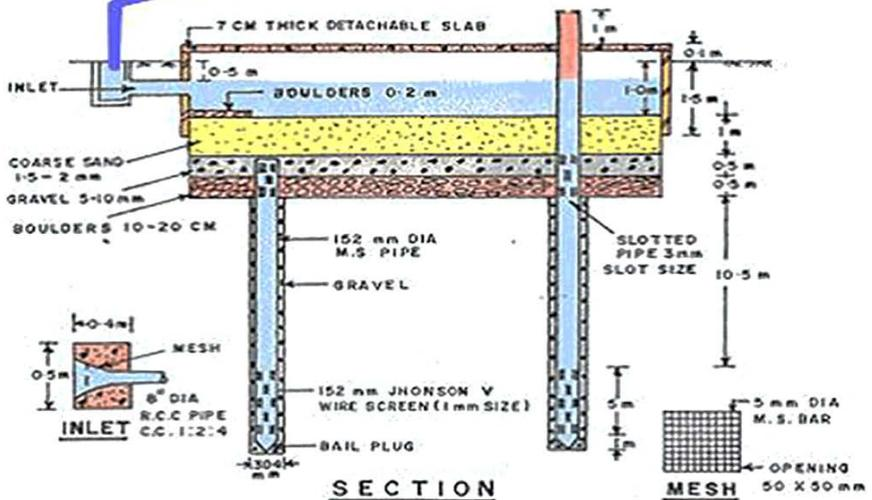
Figure (4.5): Rooftop rainwater harvesting through trench with recharge wells [14]
