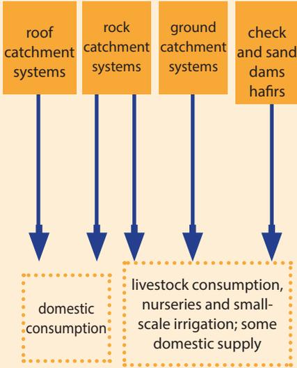
Figure (2.1): Water harvesting systems and their uses[6]
