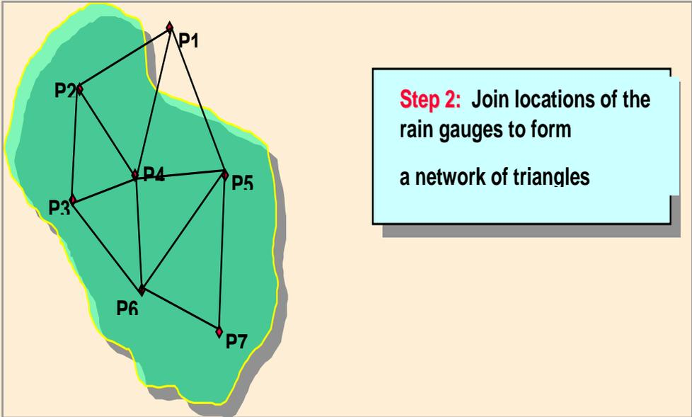
**Step 2:** Join locations of the rain gauges to form a network of triangles
