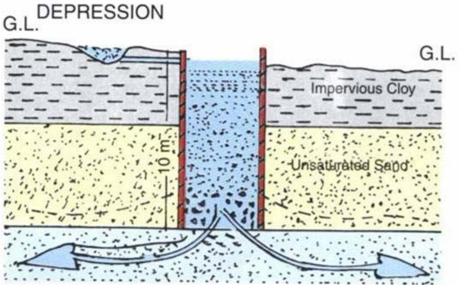
Figure (4.9): Rainwater harvesting from roof through shaft without injection well
