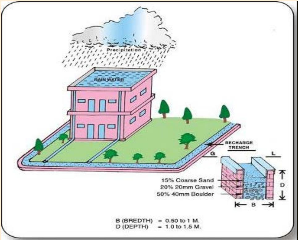
Figure (4.3): Rainwater harvesting recharge trench [14]
