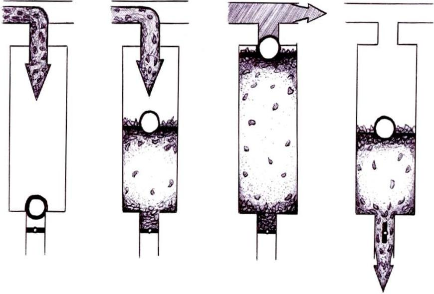
1. This is what the pre-filter looks like during the dry season before the first rains come. It is empty and dry having been flushed out at the end of the previous rainy season. It is important to drain and dry this out to prevent mosquitoes from breeding. The pre-filter chamber is sized large enough to allow the debris-laden water to flush the roof, gutters and downspout and settle here without entering the storage tank.
