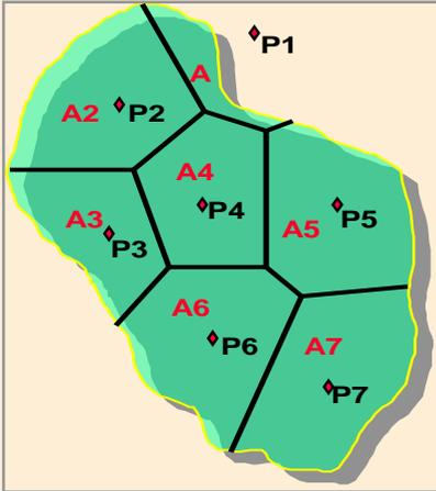
**Step 4:** Delineate the formed polygons and measure their areas using a planimeter or by converting them into smaller regular geometric shapes (i.e. triangles, squares, rectangles, etc.)
