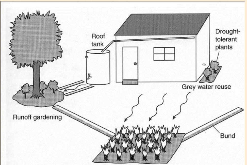
Figure (5.1): General roof catchments and harvesting water uses [7]
