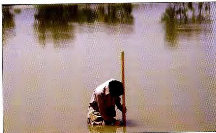
FIGURE 25. DEPTH OF WATER APPLIED TO BUNDRA DURING FLOOD IRRIGATION
